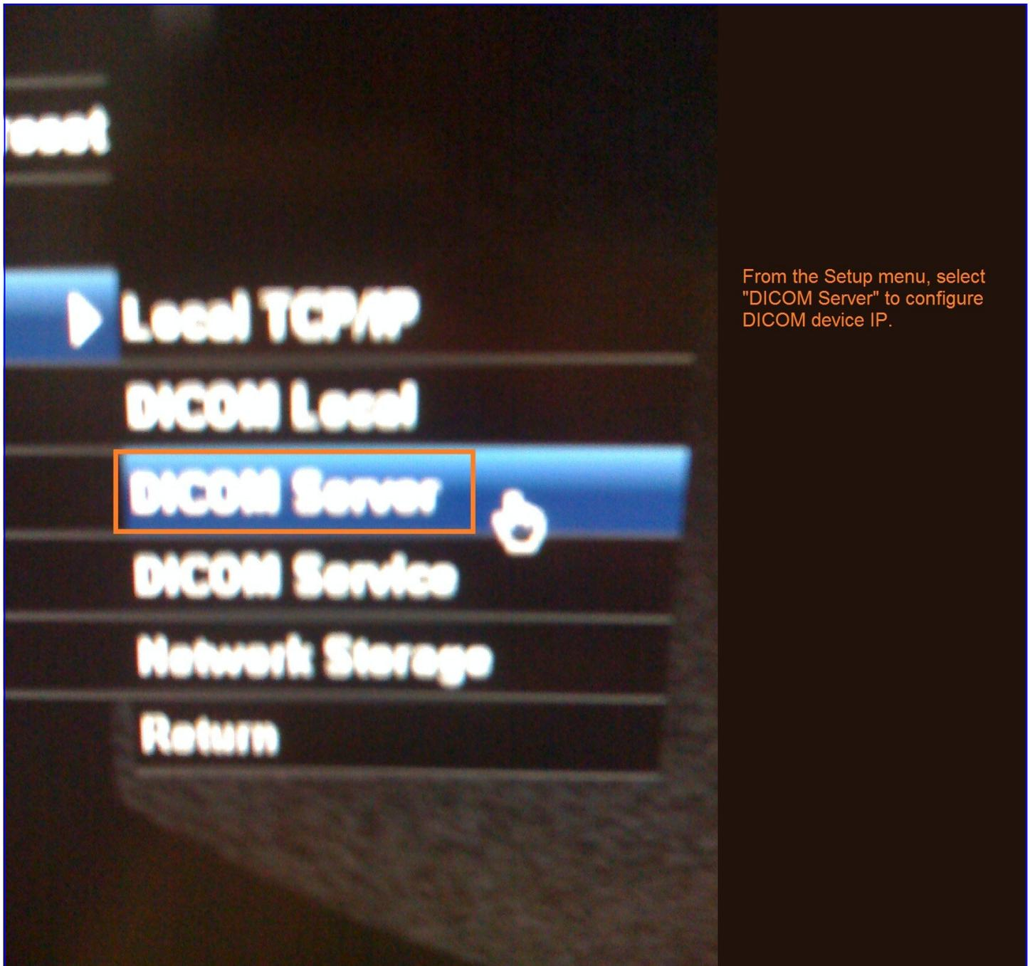
From the Setup menu, select "DICOM Server" to configure DICOM device IP.
