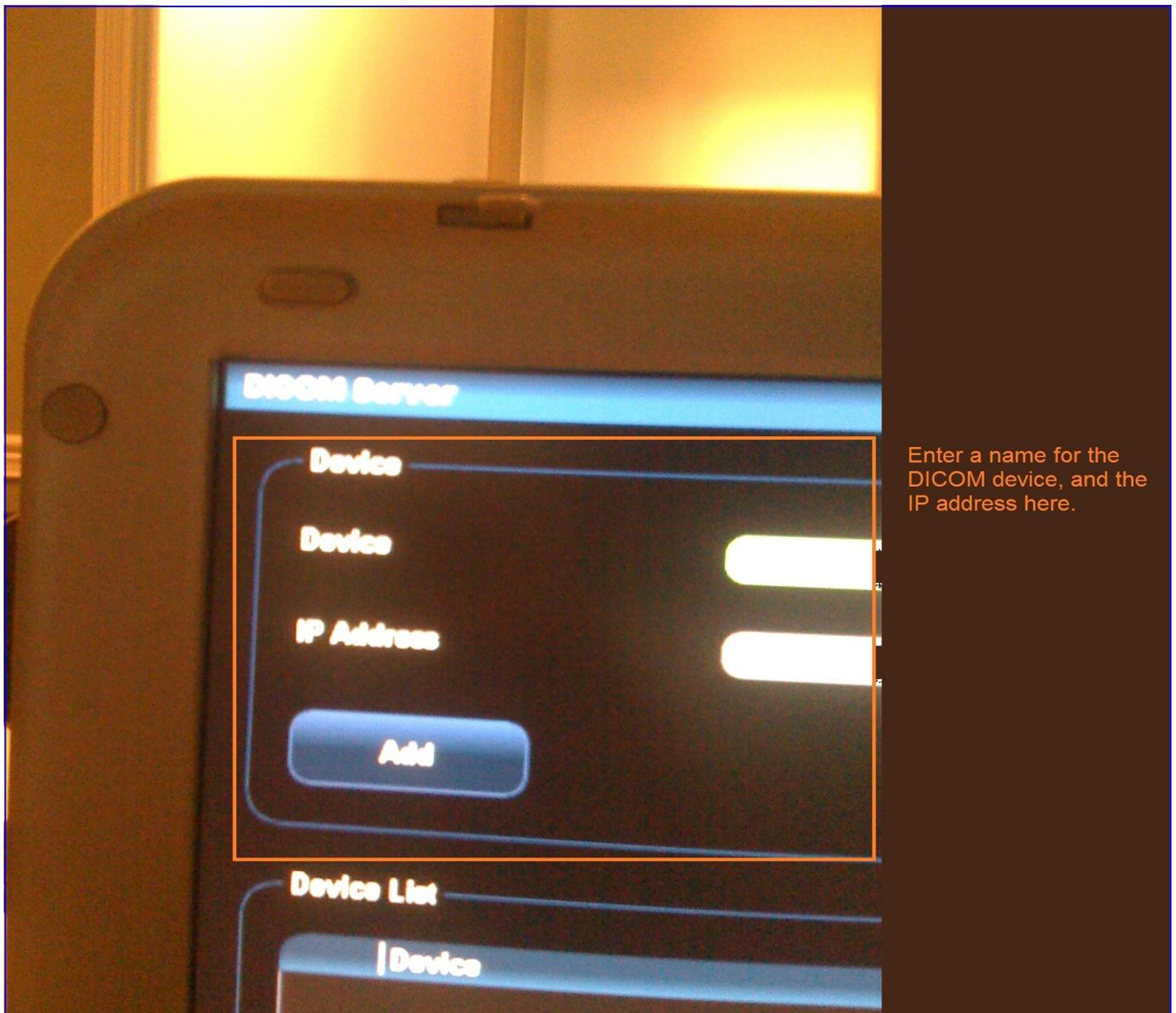
Enter a name for the DICOM device, and the IP address here.
